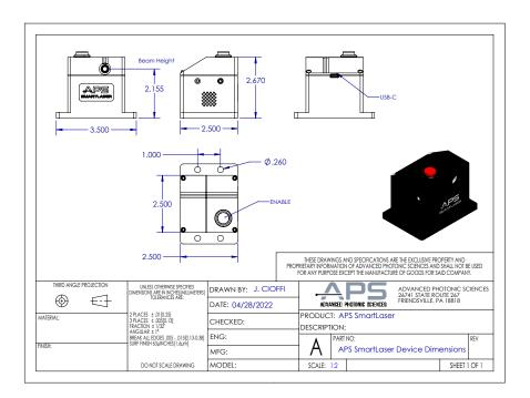
Figure 4: SmartLaser Device Dimensions
