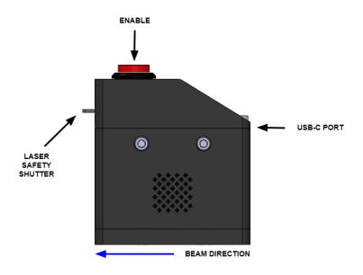
Figure 1: Standard Operation
