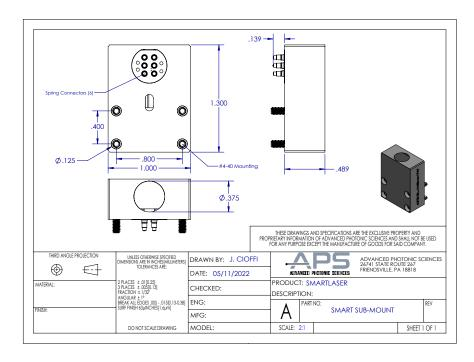
Figure 5: Replaceable Smart Sub-Mount Dimensions
